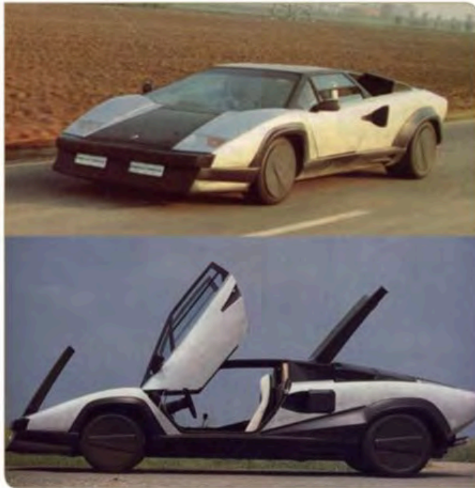
Fig.1: 1986 the Countach Evoluzione : the dream of an all CFRP Lamborghini car
